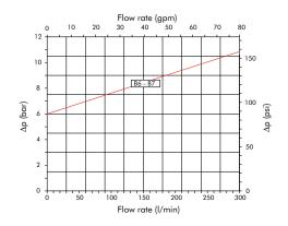
The above diagrams have been obtained at the FILTREC laboratory, according to the ISO 3968 specification, with mineral oil having 30 cSt viscosity and 0,86 Kg/dm3 density.
